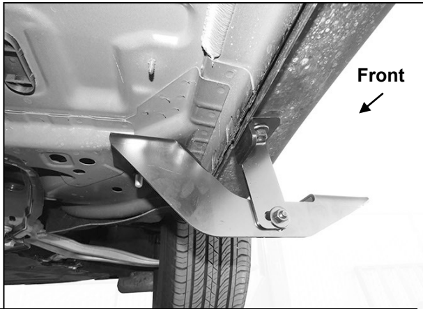
(Fig 16) Passenger/right front Mounting Brackets installed
